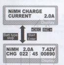
This program simply charges the battery using the current you set. The charge current ranges from 0.1 to 5.0A.
